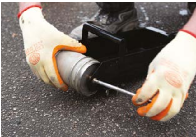
5. Replace the drum and spindle once clean and retain back in place with the split pin.
