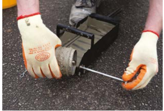
2. When you're done with the roller, simply remove the split pin and spindle to release the drum.
