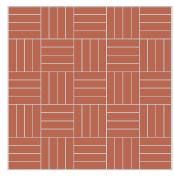
**Basket Weave**Using WF format clay pavers (200x48x85mm)
