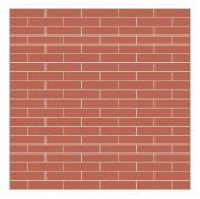
**Stretcher Bond**Using WF format clay pavers (200x48x85mm)
