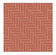
**90° Herringbone**Using WF format clay pavers (200x48x85mm)
