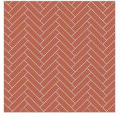
**45° Herringbone**Using WF format clay pavers (200x48x85mm)
