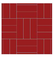
**Basket Weave**Using DF format clay pavers (200x64x85mm)
