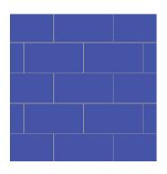
**Stretcher Bond**Using rectangular clay pavers (200x100)
