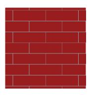
**Stretcher Bond**Using DF format clay pavers (200x64x85mm)
