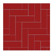
**90° Herringbone**Using DF format clay pavers (200x64x85mm)
