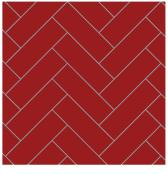
**45° Herringbone**Using DF format clay pavers (200x64x85mm)
