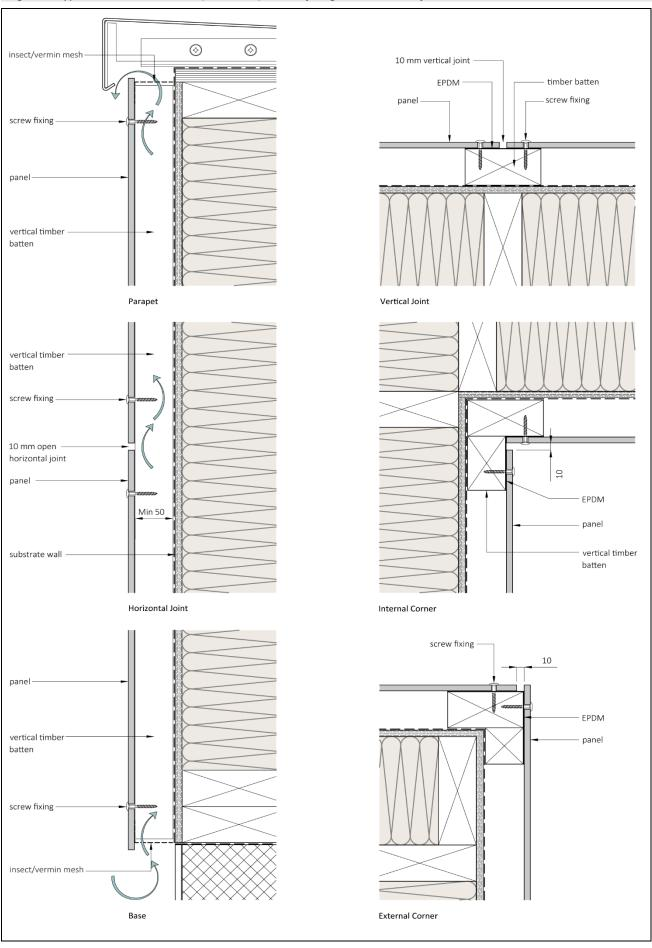
Figure 3 Typical installation details (continued) - screw fixing and timber subframe
