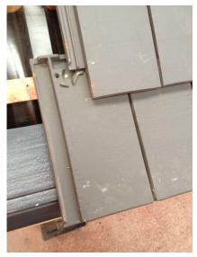
The side interlock on the standard Vauban tile stops 70mm short of the tail, therefore special eaves course tiles are required which have extended side interlocks. These will be available at the same price as the standard tiles.
