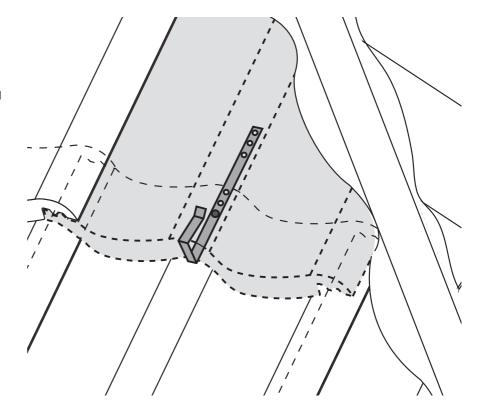
2. Where it is not possible to secure the clip through the nail hole of the tile below (because it has been removed in cutting) then the clip can be secured by bending it over the head of the tile below.
