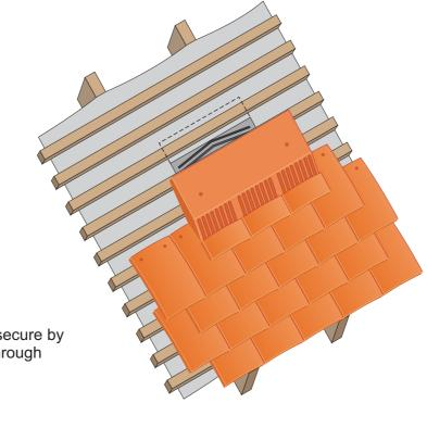
Position ventilator and secure by nailing into tile batten through holes provided.
