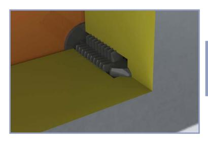
Cavity insulation fixings
