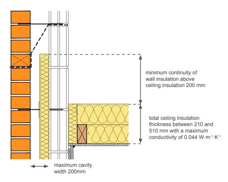
This indicative guidance illustrates good practice for design and construction with respect to achieving thermal performance and air barrier continuity only. It must be implemented taking due regard of site conditions and all other requirements imposed by Buiding Regulations.
