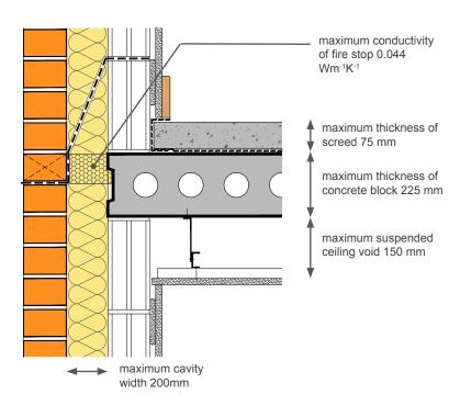
This indicative guidance illustrates good practice for design and construction with respect to achieving thermal performance and air barrier continuity only. It must be implemented taking due regard of site conditions and all other requirements imposed by Building Regulations.
