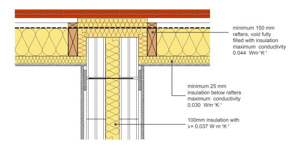
This indicative guidance illustrates good practice for design and construction with respect to achieving thermal performance and air barrier continuity only. It must be implemented taking due regard of site conditions and all other requirements imposed by Building Regulations.
