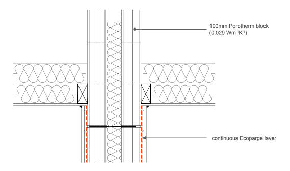
This indicative guidance illustrates good practice for design and construction with respect to achieving thermal performance and air barrier continuity only. It must be implemented taking due regard of site conditions and all other requirements imposed by Building Regulations.
