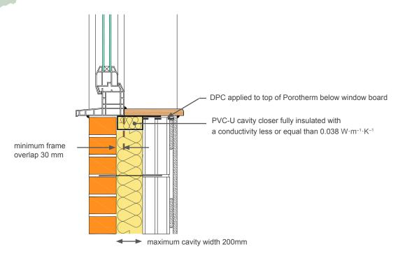
This indicative guidance illustrates good practice for design and construction with respect to achieving thermal performance and air barrier continuity only. It must be implemented taking due regard of site conditions and all other requirements imposed by Building Regulations.
