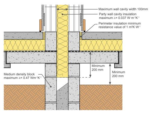
This indicative guidance illustrates good practice for design and construction with respect to achieving thermal performance and air barrier continuity only. It must be implemented taking due regard of site conditions and all other requirements imposed by Buiding Regulations.
