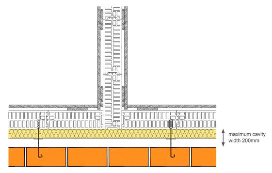
This indicative guidance illustrates good practice for design and construction with respect to achieving thermal performance and air barrier continuity only. It must be implemented taking due regard of site conditions and all other requirements imposed by Buiding Regulations.
