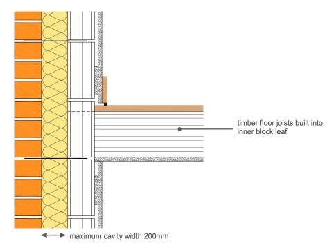
This indicative guidance illustrates good practice for design and construction with respect to achieving thermal performance and air barrier continuity only. It must be implemented taking due regard of site conditions and all other requirements imposed by Building Regulations.
