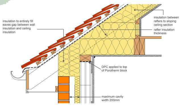
This indicative guidance illustrates good practice for design and construction with respect to achieving thermal performance and air barrier continuity only. It must be implemented taking due regard of site conditions and all other requirements imposed by Buiding Regulations.
