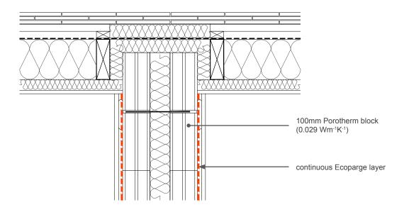
This indicative guidance illustrates good practice for design and construction with respect to achieving thermal performance and air barrier continuity only. It must be implemented taking due regard of site conditions and all other requirements imposed by Building Regulations.
