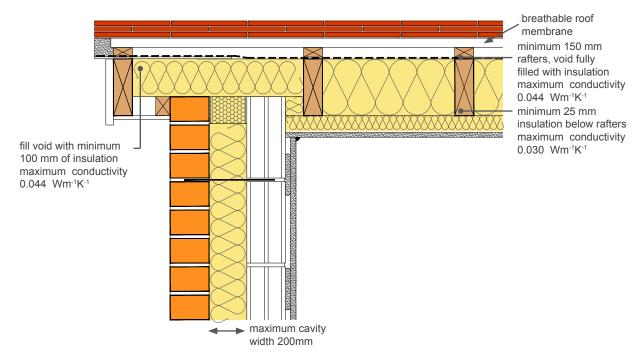
This indicative guidance illustrates good practice for design and construction with respect to achieving thermal performance and air barrier continuity only. It must be implemented taking due regard of site conditions and all other requirements imposed by Building Regulations.
