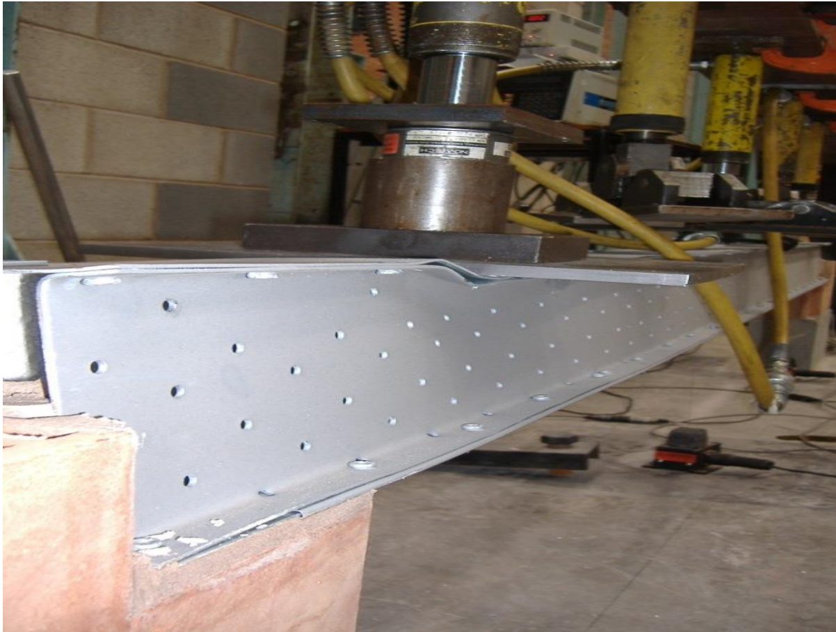
Figure H3: Localised Failure of Lintel due to Shear Load
