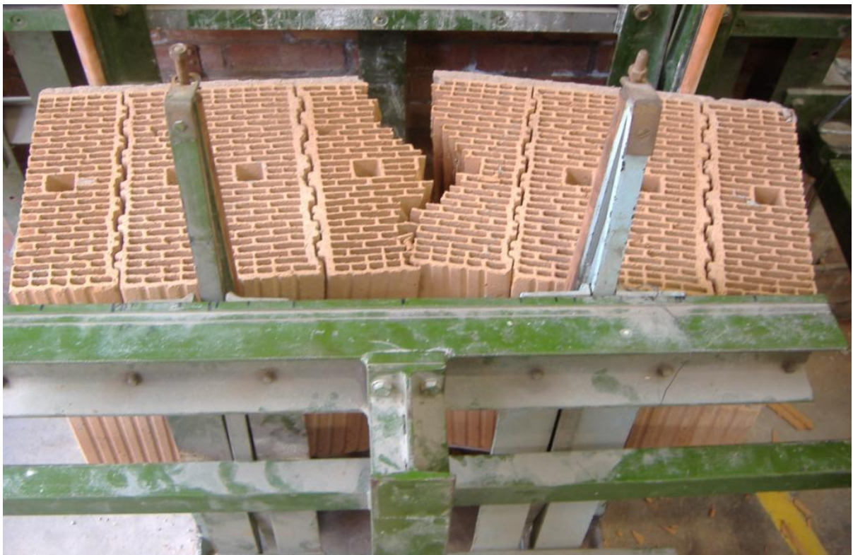
Figure H2: Flexural Failure of 365 mm Porotherm Blockwork
