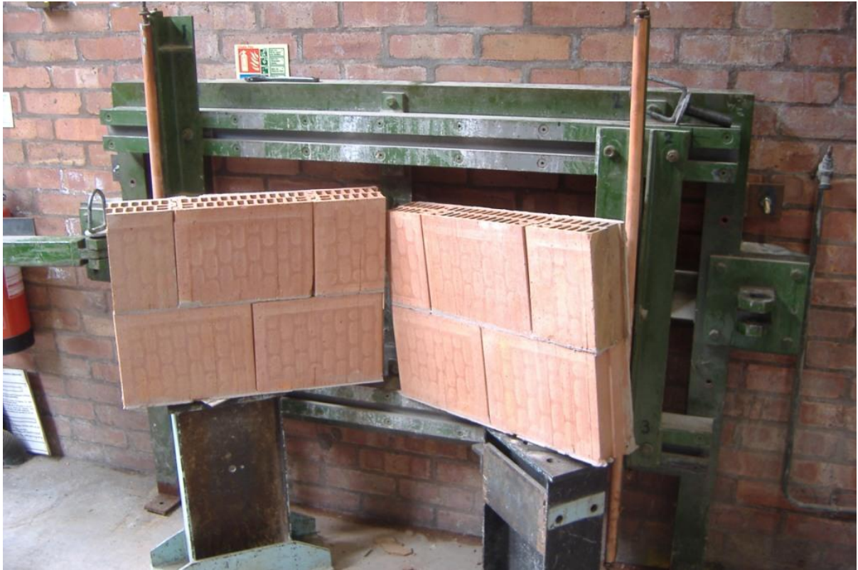
Figure H1: Flexural Failure of 100 mm Porotherm Blockwork
