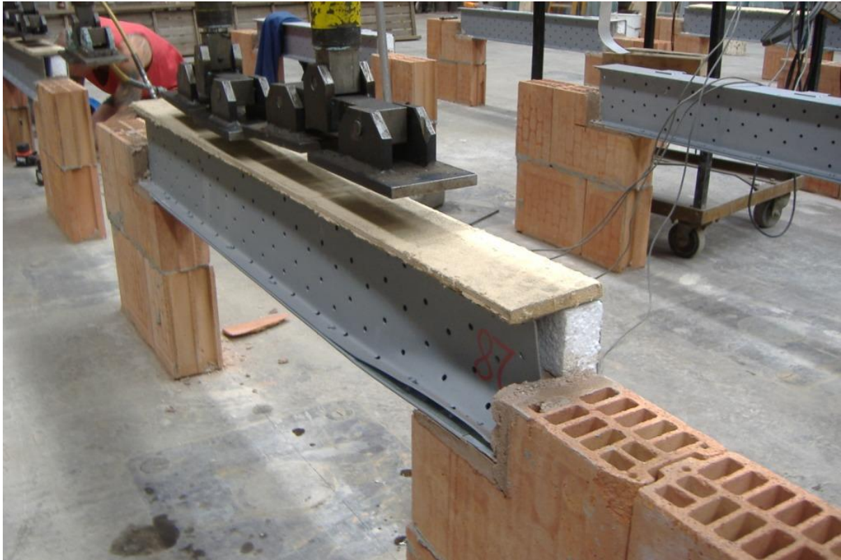
Figure H5: Localised Buckling of Lintel Web in Flexural Test
