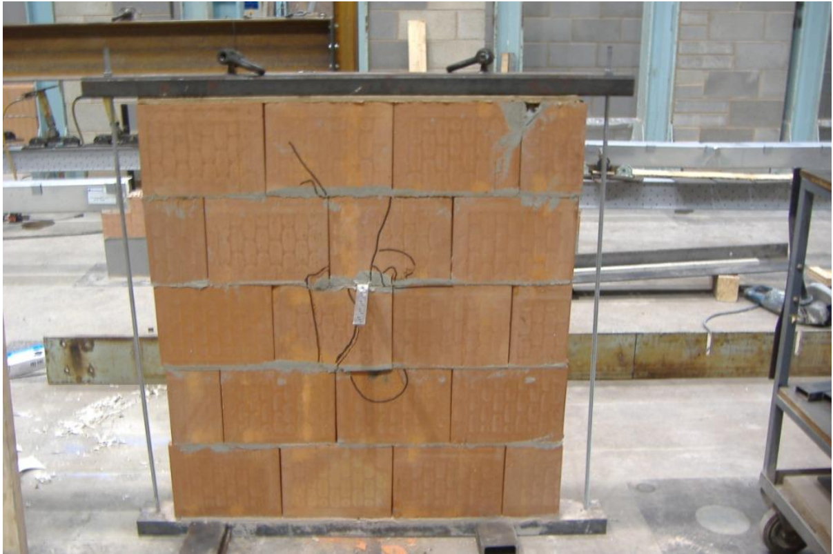
Figure H7: Failure of Horizontal Tensile Restraint Strap
