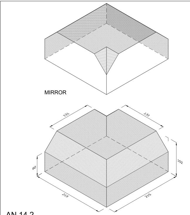
AN.14.2 DOUBLE CANT EXTERNAL RETURN WITH INTERNAL MITRE (SCOB)
